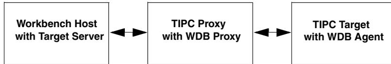
The Workbench host communicates using UDP, the TIPC target communicates using TIPC, and the proxy translates between them.
