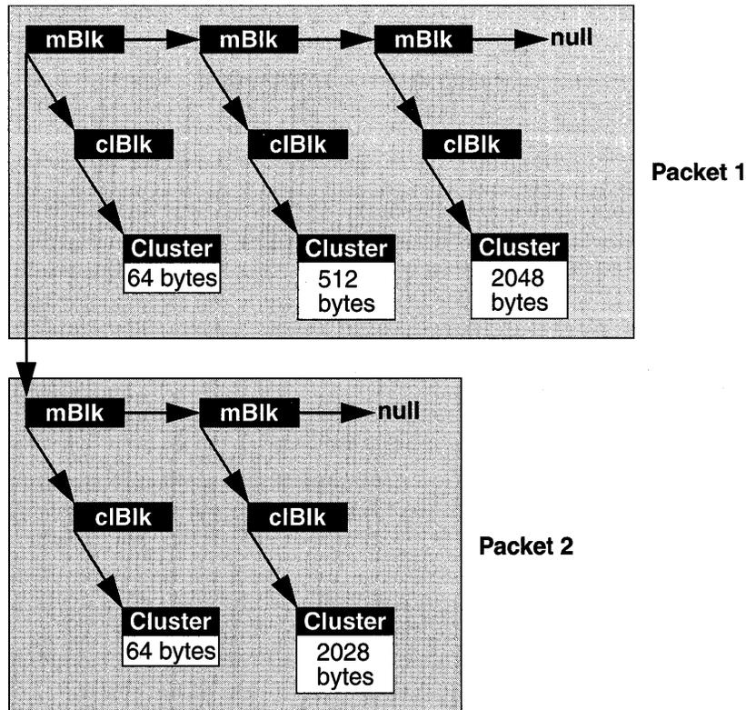
As shown in Figure 4-5, an **mBlk** references data only indirectly – through a **cBlk** structure. This indirection makes it easier for multiple **mBlks** to share the same cluster. See Figure 4-6.
